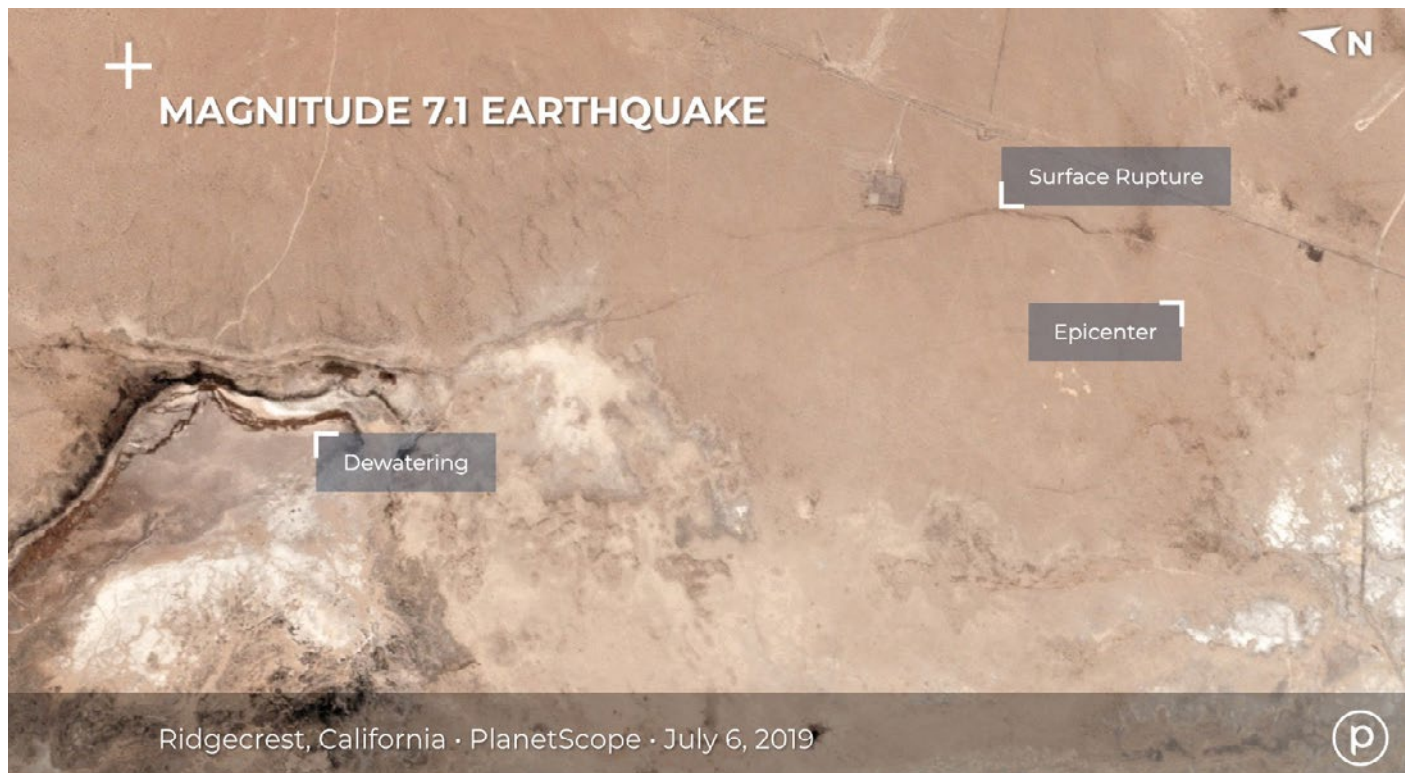
PlanetScope view of a surface rupture and dewatering from the M_w 7.1 earthquake discussed by Milliner and Donnellan (2020).
