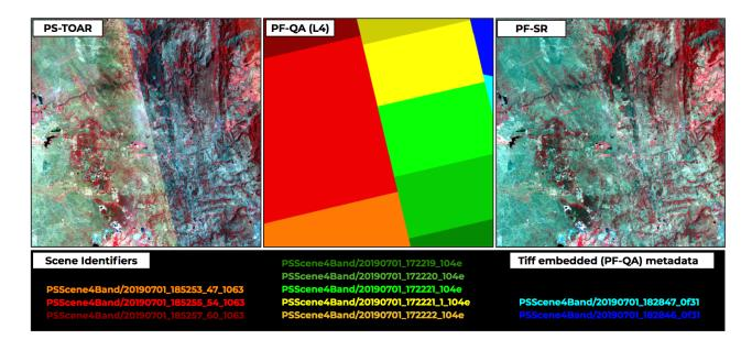
QA layer 5 (Table 5) identifies the number of FLS-SR scenes (i.e., Sentinel-2 or Landsat 8) used for each pixel during reference sampling and CESTEM calibration. In general the larger the number of reference scenes, the more robust the calibration is expected to be (see Section 4.3).
