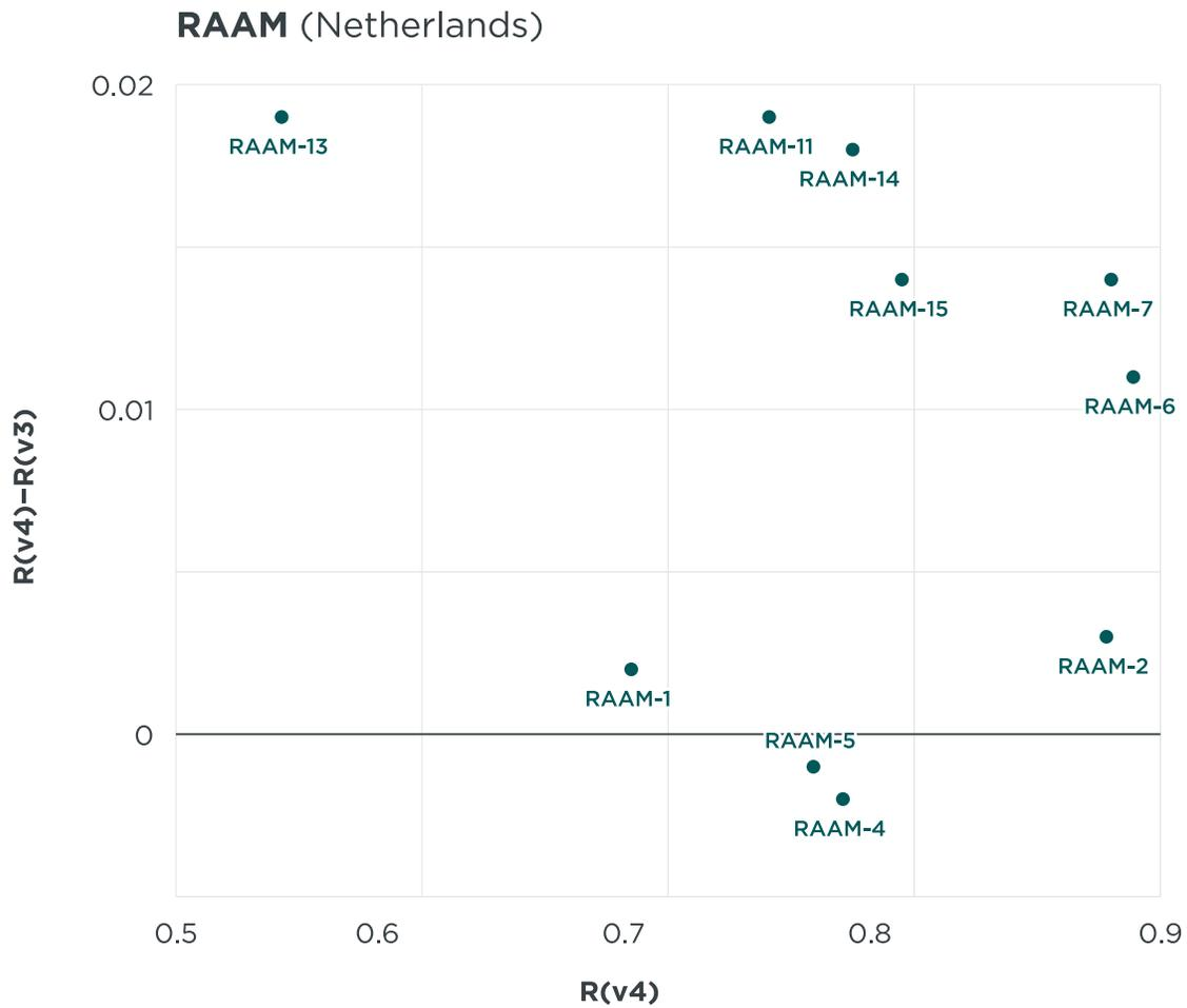
**Figure 12:** Correlation coefficients of L-band SWC version 4 and the difference with version 3 for each sensor in the RAAM network.
