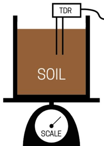
**Figure A.2:** A schematic representation of a setup where both the soil weight and the sensor reading can be obtained.
