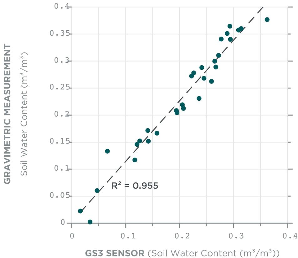
**FigureA.3:** An example of a scatter plot between SWC readings as given by the FDR sensor and the measured SWC based on the measured sample weights.
