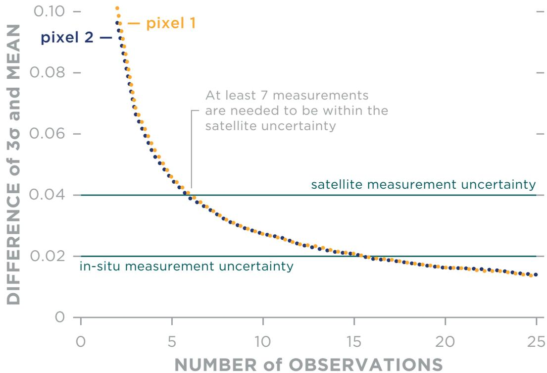
**Figure 9:** Difference between  $3\sigma$  and mean of the observation pairs with a certain number of in-situ observations
