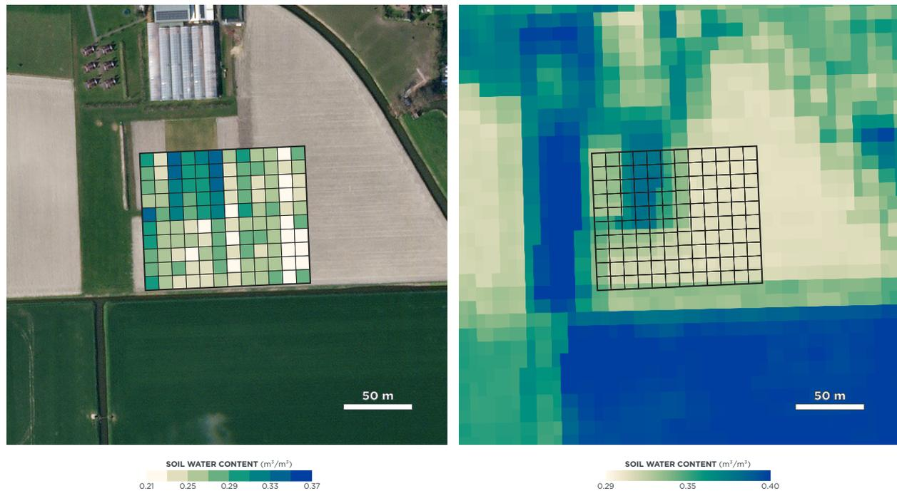
**Figure 8:** Spatial maps of SWC from TDR sensors( left), representing more than 1,100 measurements vs. 10 m L-band ER (right).
