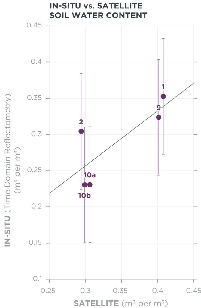
**Figure 7:** L-band SWC 10 m vs. in-situ TDR SWC, including field numbers
