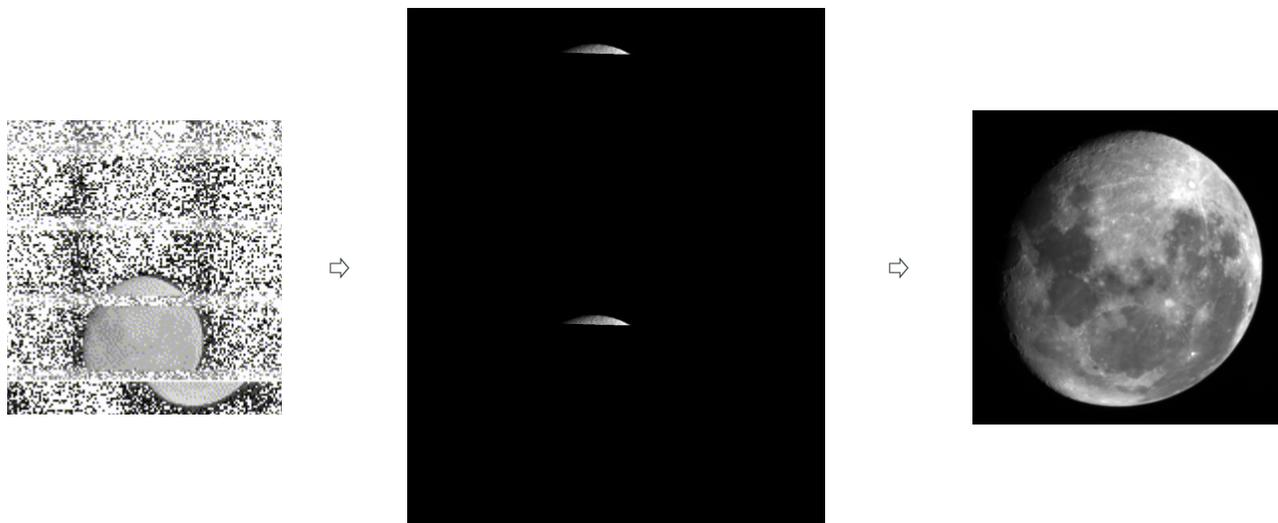
Once lunar images are collected, reconstructed, stored and analyzed for determining the measured lunar radiance, the ROLO model radiance is calculated based on the relative geometry of the Earth, moon and satellite at the time images were collected (Figure 13).
