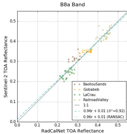
Figure 21: Example validation: SkySat s4 sensor 2 TOA reflectance compared to RadCalNet calibration site data for the Sentinel-2 spectral bands. The corresponding results for Sentinel-2 TOA reflectance, collected over the same time period, are shown on the right for comparison.
