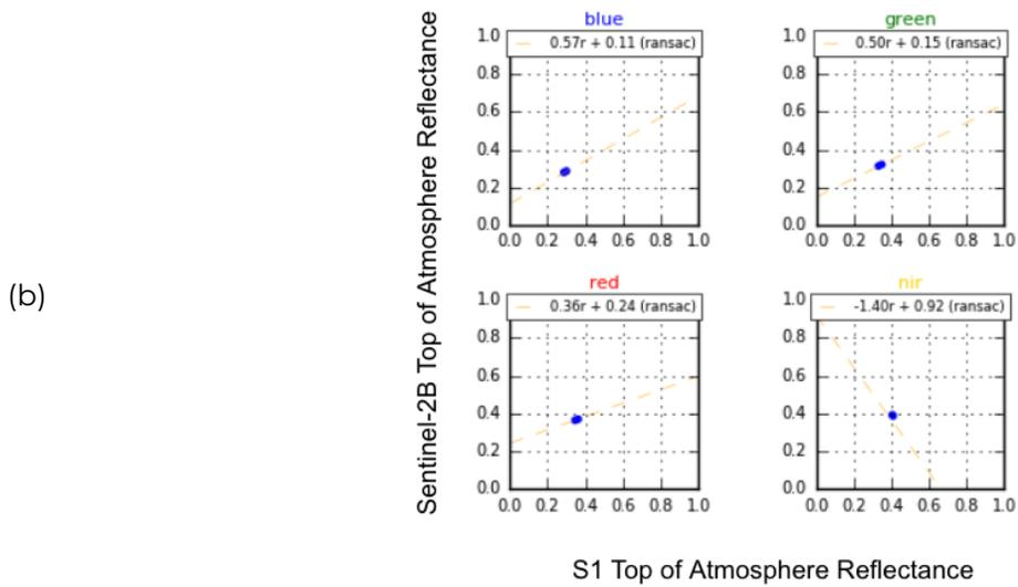
Figure 7: A single crossover event between Dove Classic and Sentinel 2. Over 30 common sample areas are intersected but both satellites in this example (a). Since the region is approximately homogeneous, the sample data points all cluster tightly together (b). The joint mode is then calculated from these points.
